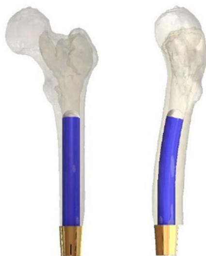
Anterior and lateral view of implant in bone. 18mm implant diameter, 120mm effective length within IM canal.
